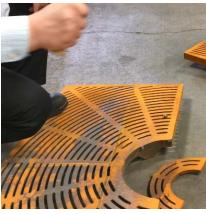
3. After several hits, the breakaway section should snap cleanly off of the larger grate section. Reinstall the grate into the Filterra grate frame. Recycle or dispose of the breakaway section per local guidelines.
