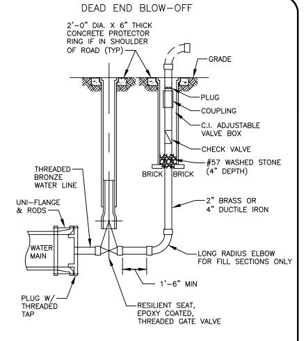
1. INSTALL 2" BLOW-OFF ON 2" THRU 8" MAINS. 2. INSTALL 2.5" BLOW-OFF ON 12" MAINS.
