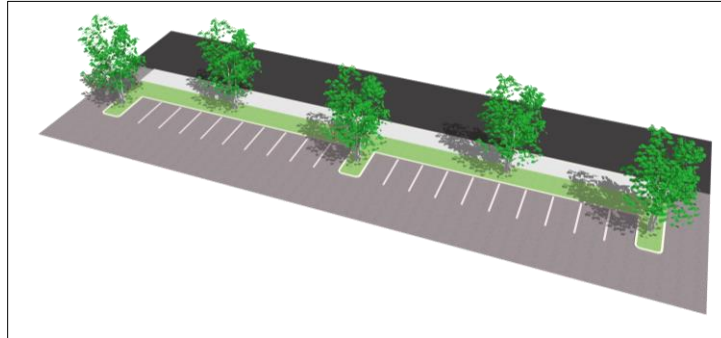
Figure 5.3.H(5)a.1(b): Interior Parking Area Minimum Plantings
