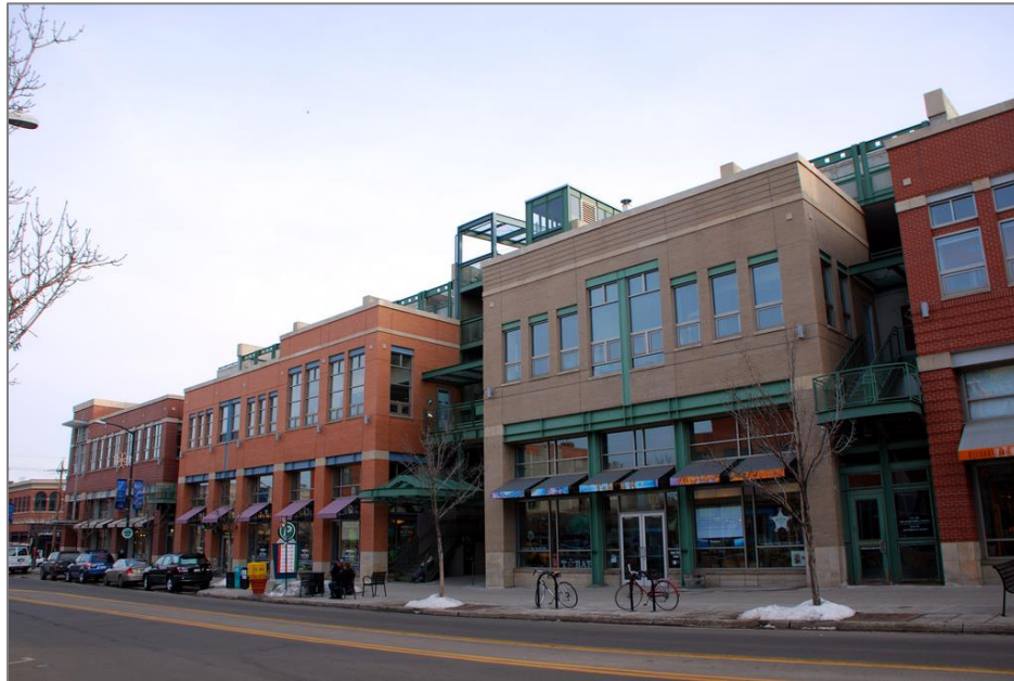
Figure 5.7.E(3)a: Example of Front Façade Offsets
