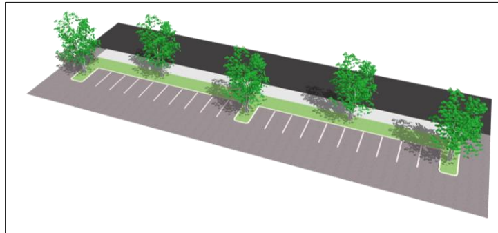
Figure 5.3.H(5)a.1(b): Interior Parking Area Minimum Plantings
